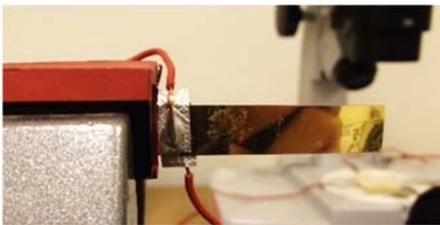
**Figure 1:** The displacement of the PVdF strip was measured in the shown configuration. Conductive adhesive tape was used for electrical connection to the two sides of the actuator. The displacement was measured using a digital microscope. In order to reduce the motion of the strip due to air current, the whole setup was placed inside a cardboard box (not shown).
